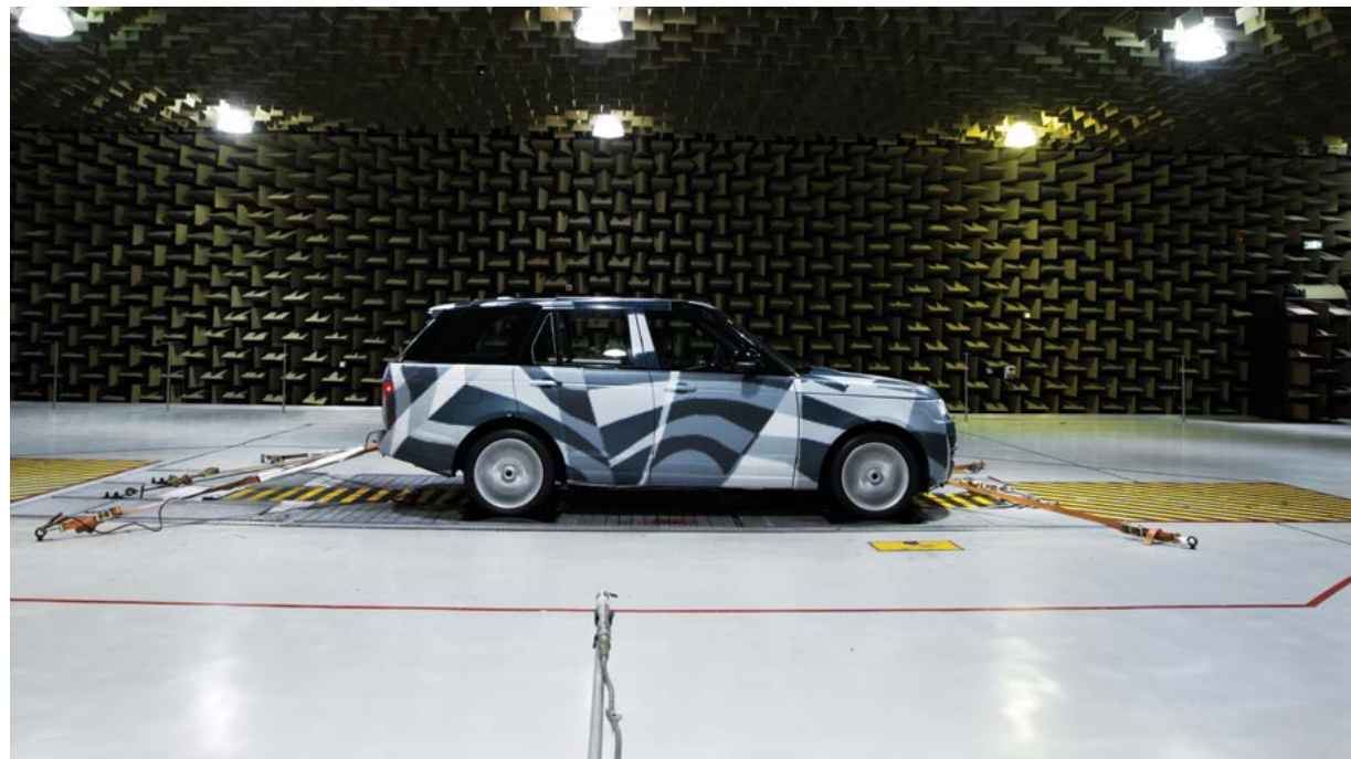
An anechoic chamber (above) and Land Rover's design studios are two of the key facilities located at Gaydon
