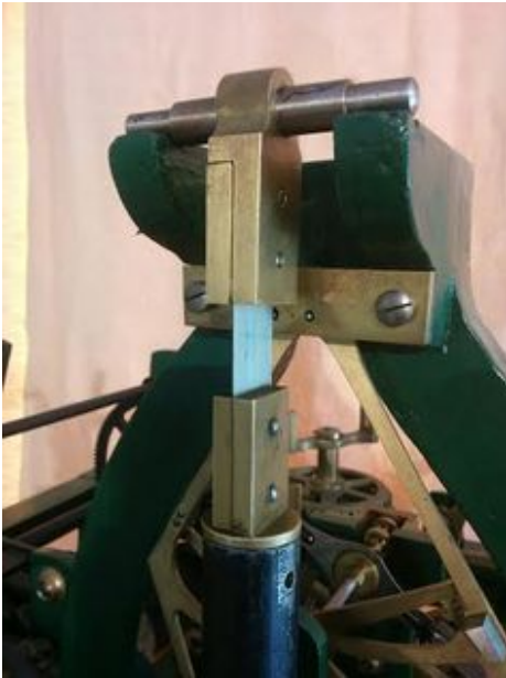
Pendulum suspension from a Smith of Derby clock. Hugh Hunt, Author provided
