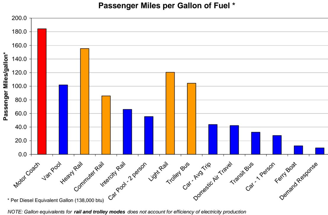
Figure 1.1 Passenger-Miles per Gallon of Fuel, by Mode
